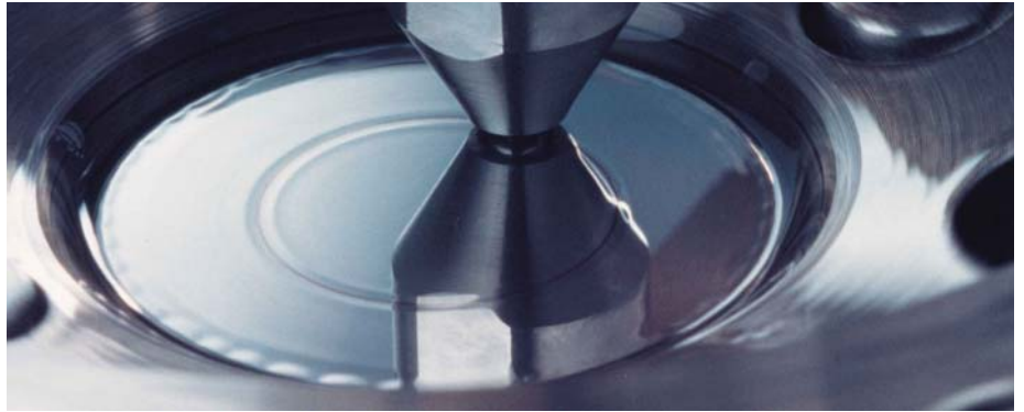
Wear test of a thin DLC layer.
