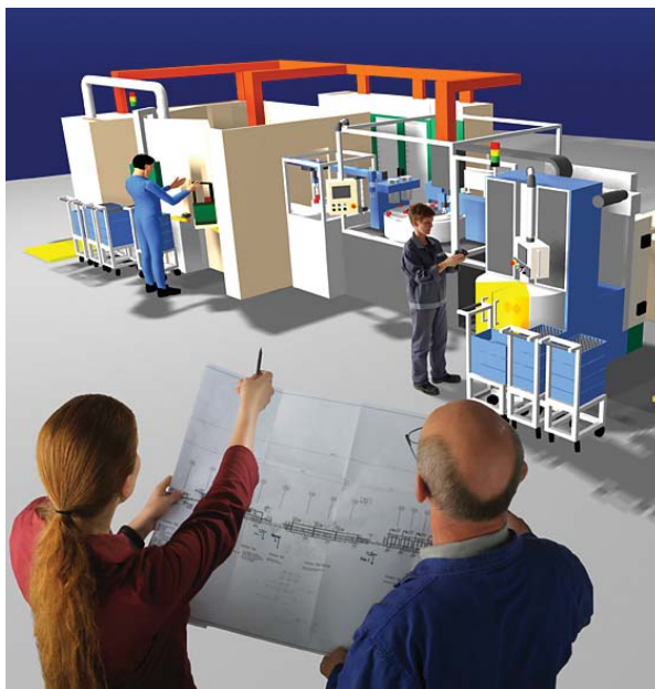
The planning of production systems is analyzed and optimized on a virtual model by using simulations. Shown here is a simulation of the ergonomics of assembly workstations.
